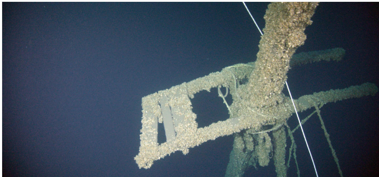
Figure 59. Tennie & Laura's foremast trestletree (Marine Imaging Technologies)
