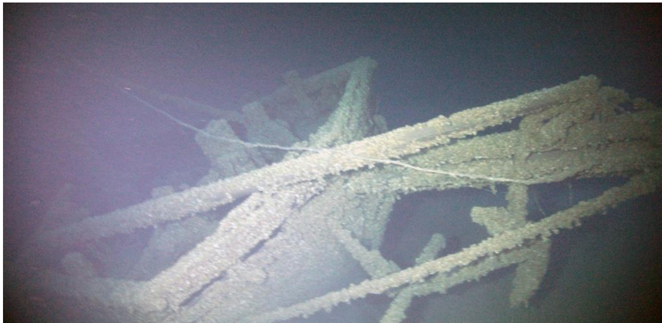
Figure 55. Tennie & Laura's V-shaped bow, windlass, jibboom, and anchor (Marine Imaging Technologies)
