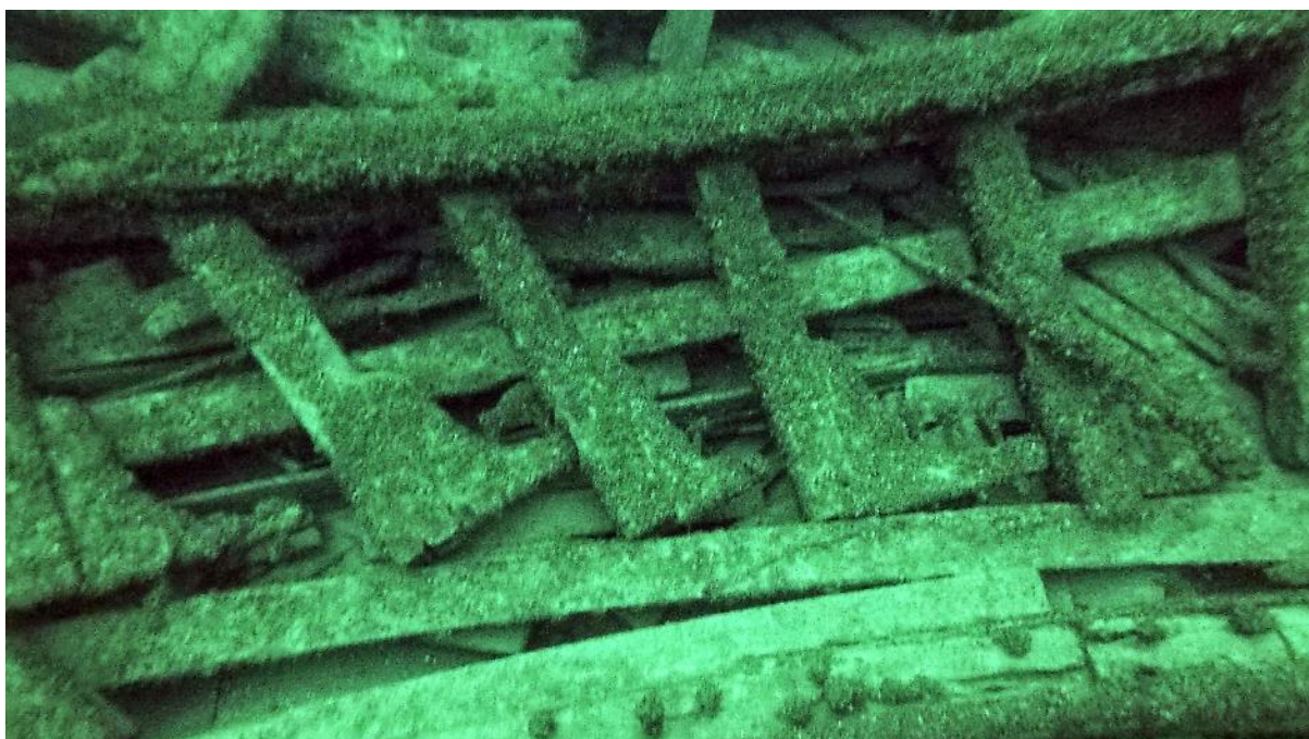
Figure 39. Transfer's stanchions with support knees (Tori Galloway)
