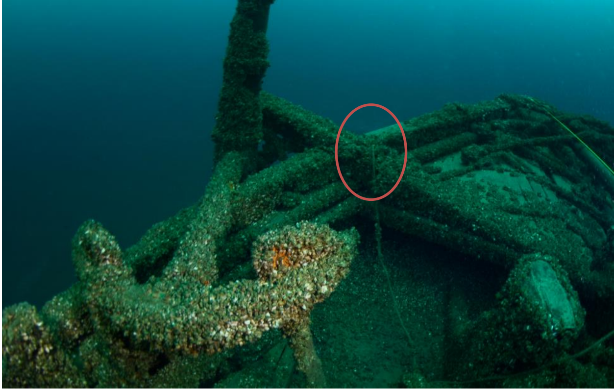
Figure 21. Grace A. Channon 's port side folding cathead with hinge (Wisconsin Historical Society).
