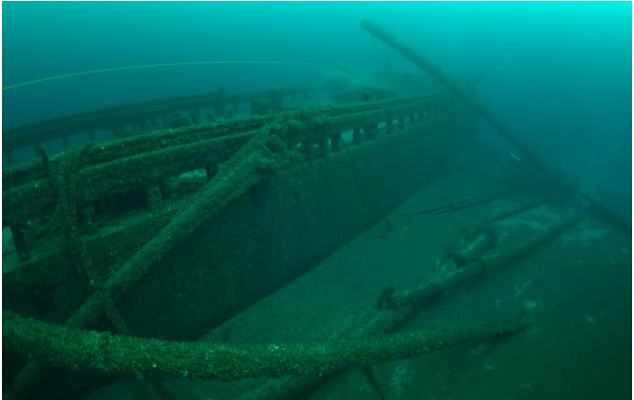
Figure 19. Grace A. Channon 's starboard side, looking forward. Note the vertical sides of the hull (Wisconsin Historical Society).
