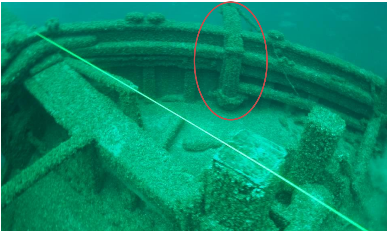
Figure 27. L-shaped catheads at Walter B. Allen 's bow (Wisconsin Historical Society).
