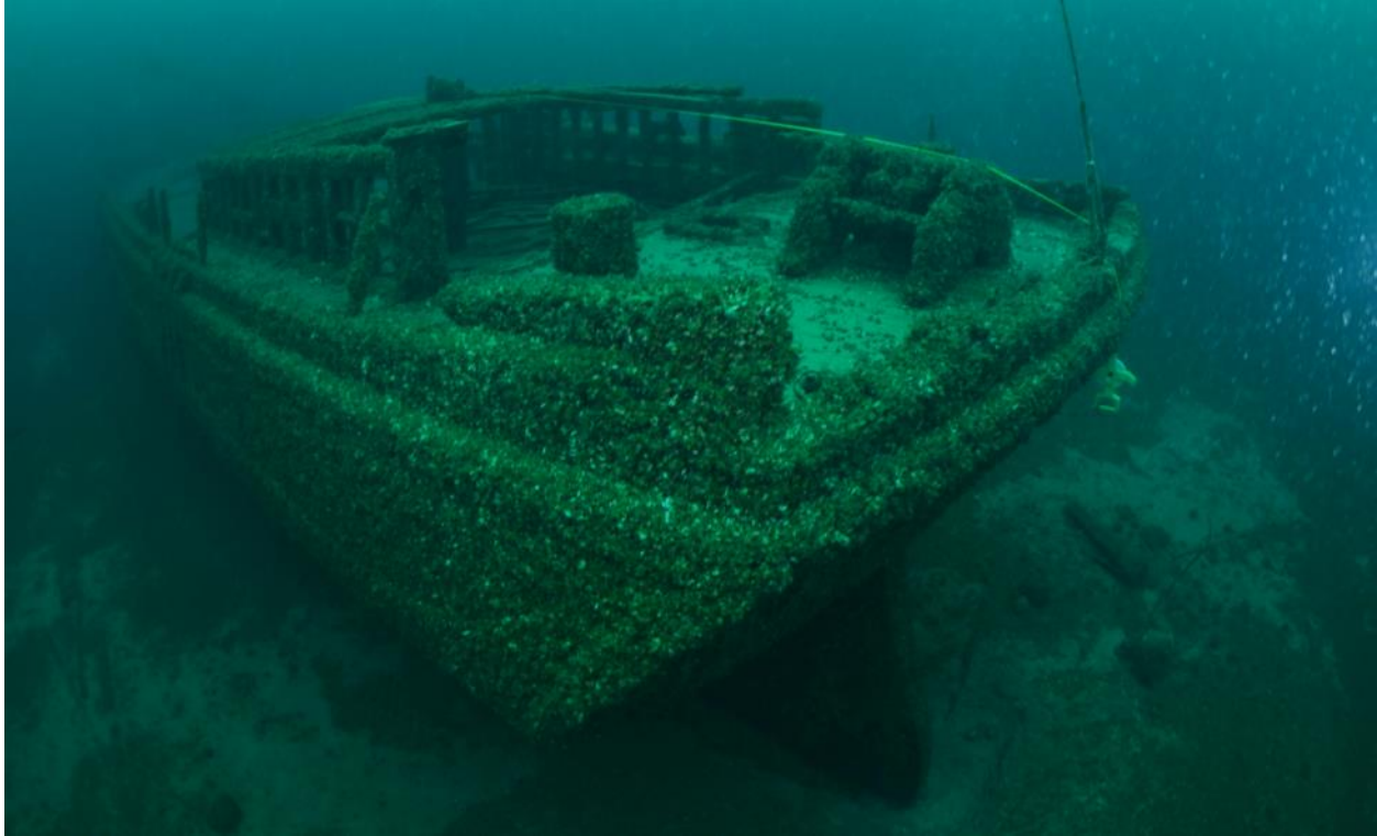
Figure 22. Grace A. Channon 's port side folding stern davit, folded back (Wisconsin Historical Society).
