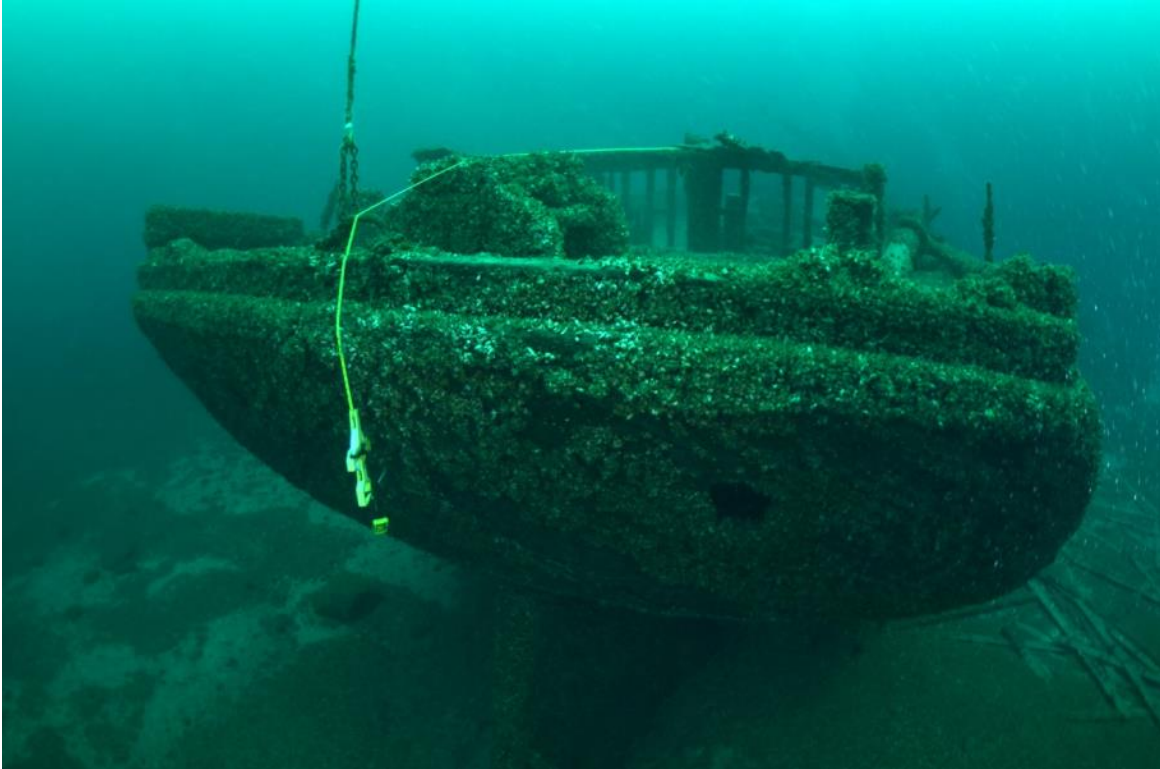
Figure 9. Photograph of Grace A. Channon 's folding stern davits (Wisconsin Historical Society).
