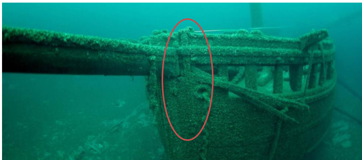
Figure 26. Walter B. Allen 's bowsprit pins (Wisconsin Historical Society).
