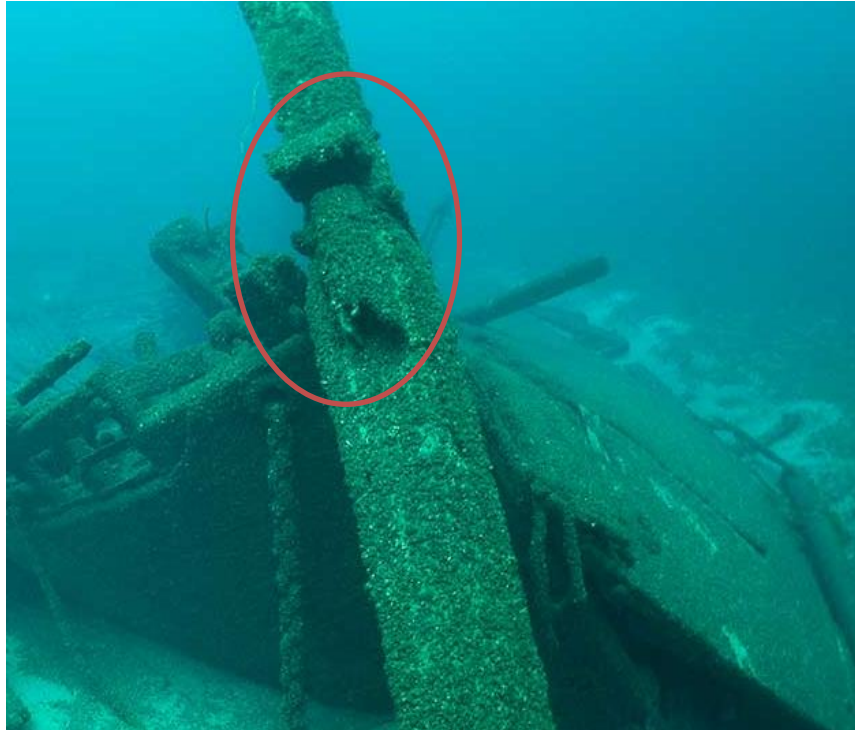
Figure 12. The rail and clamps on the stempost of America (Wisconsin Historical Society).
