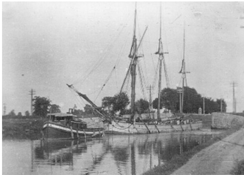
Figure 4. Image of a sailing canaller being towed out of one of the Canal locks. Note the raised bowsprit (C. Patrick Labadie Collection).
