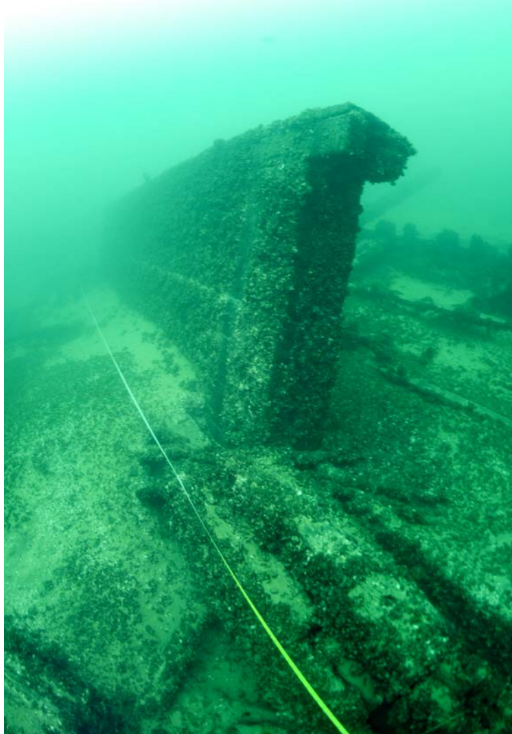
Figure 15. Advance 's standing centerboard trunk (Wisconsin Historical Society)
