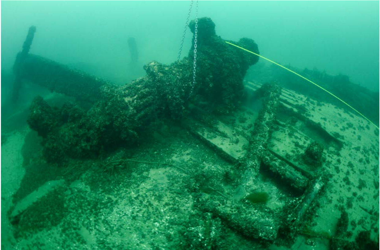
Figure 14. Advance's windlass, Samson post and deck planking (Wisconsin Historical Society)
