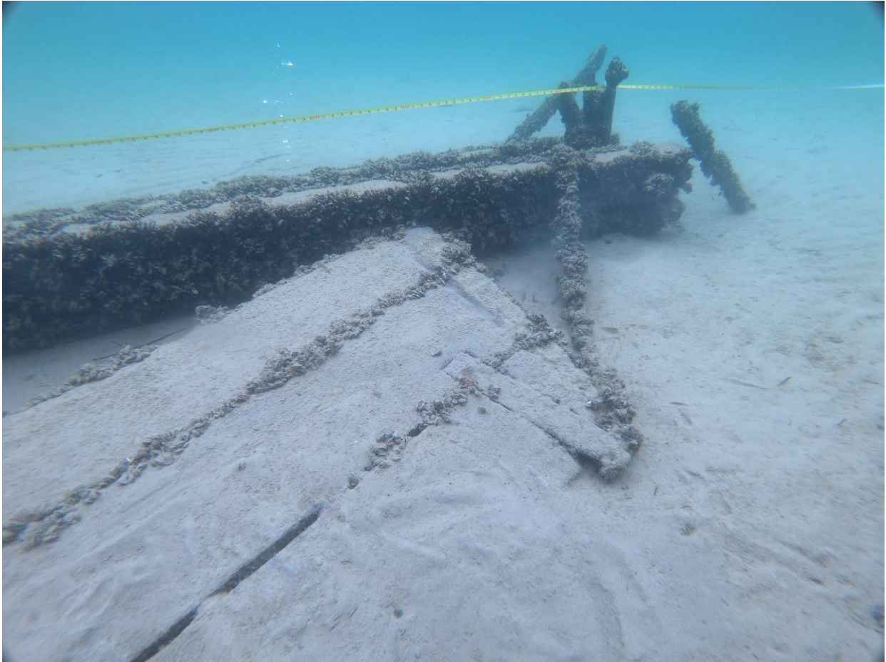
Figure 57. Sunshine 's centerboard trunk, broken centerboard, and centerboard winch chain (Wisconsin Historical Society)
