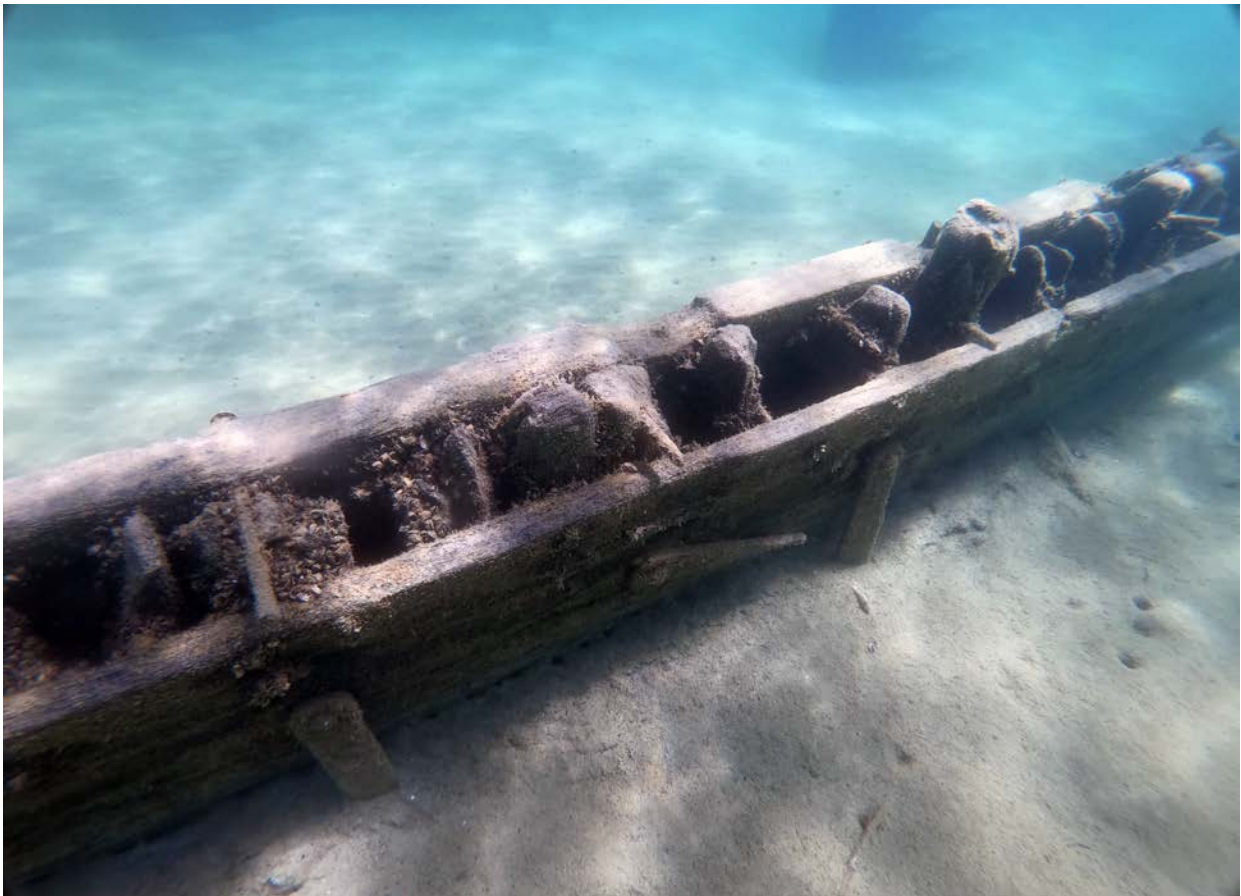
Figure 25. Peoria's portside foremast chainplates (Wisconsin Historical Society)
