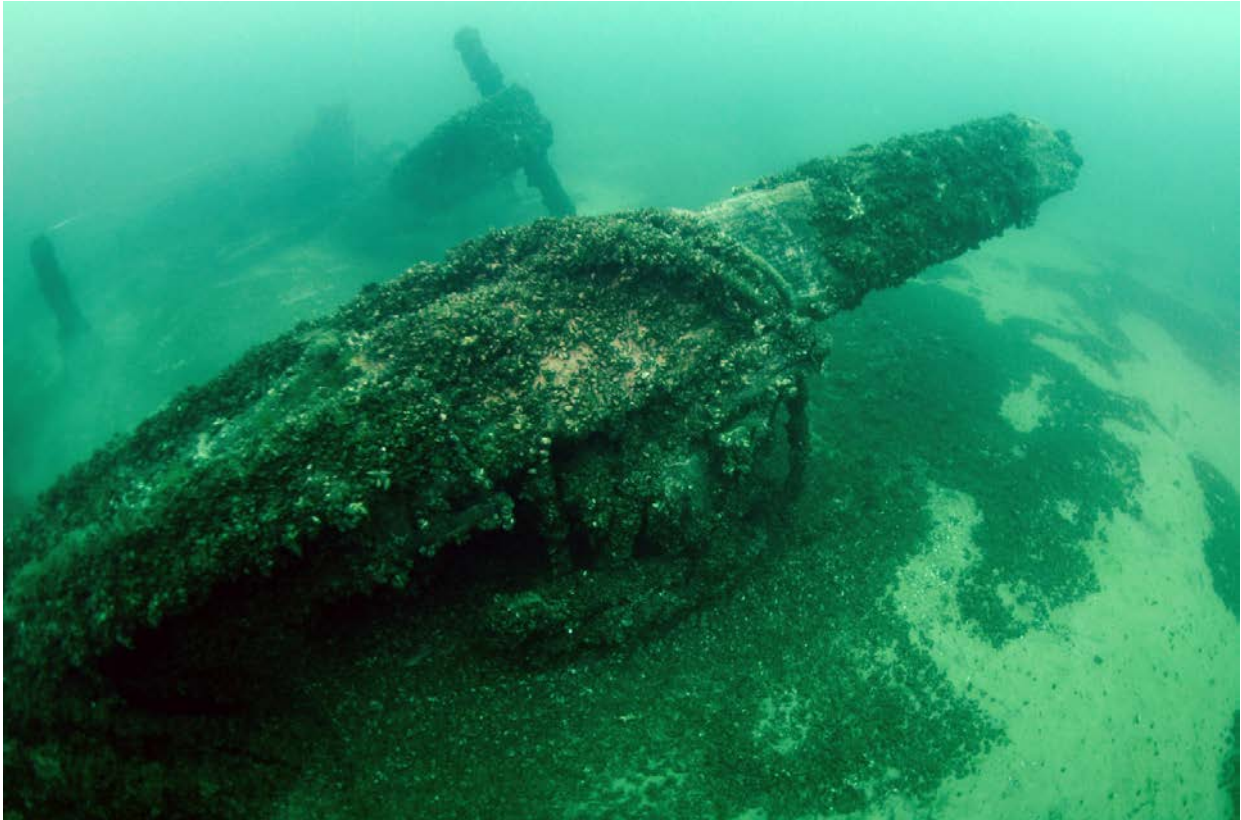
Figure 13. Bowsprit and head rigging of Advance (Wisconsin Historical Society)
