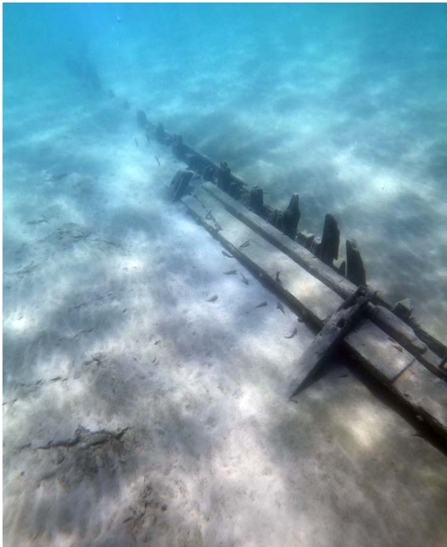
Figure 26. Peoria's portside deck shelf and two deck beams (Wisconsin Historical Society)
