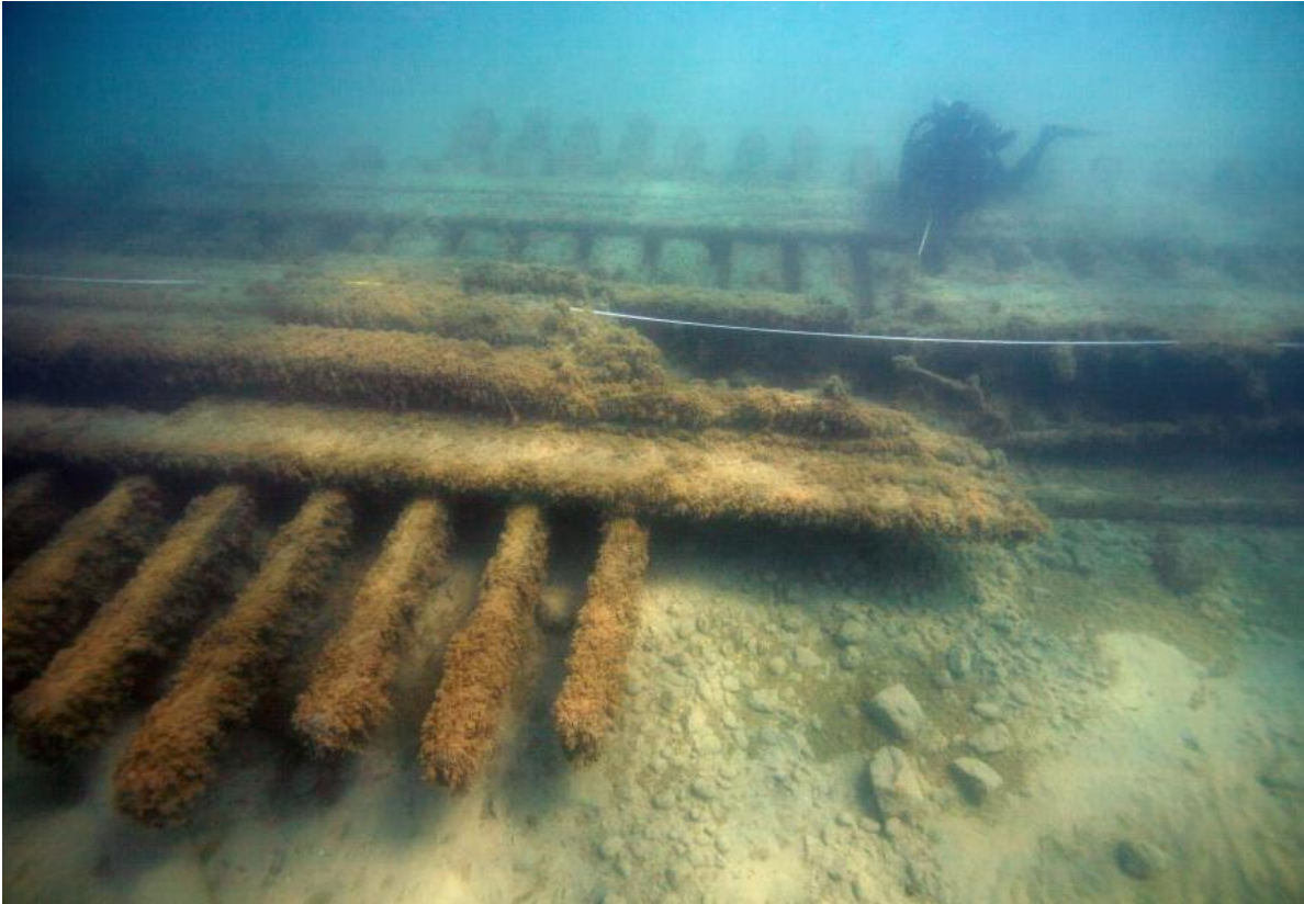
Figure 36. H.L. Whitman 's missing keel section in profile (Christa Waller)
