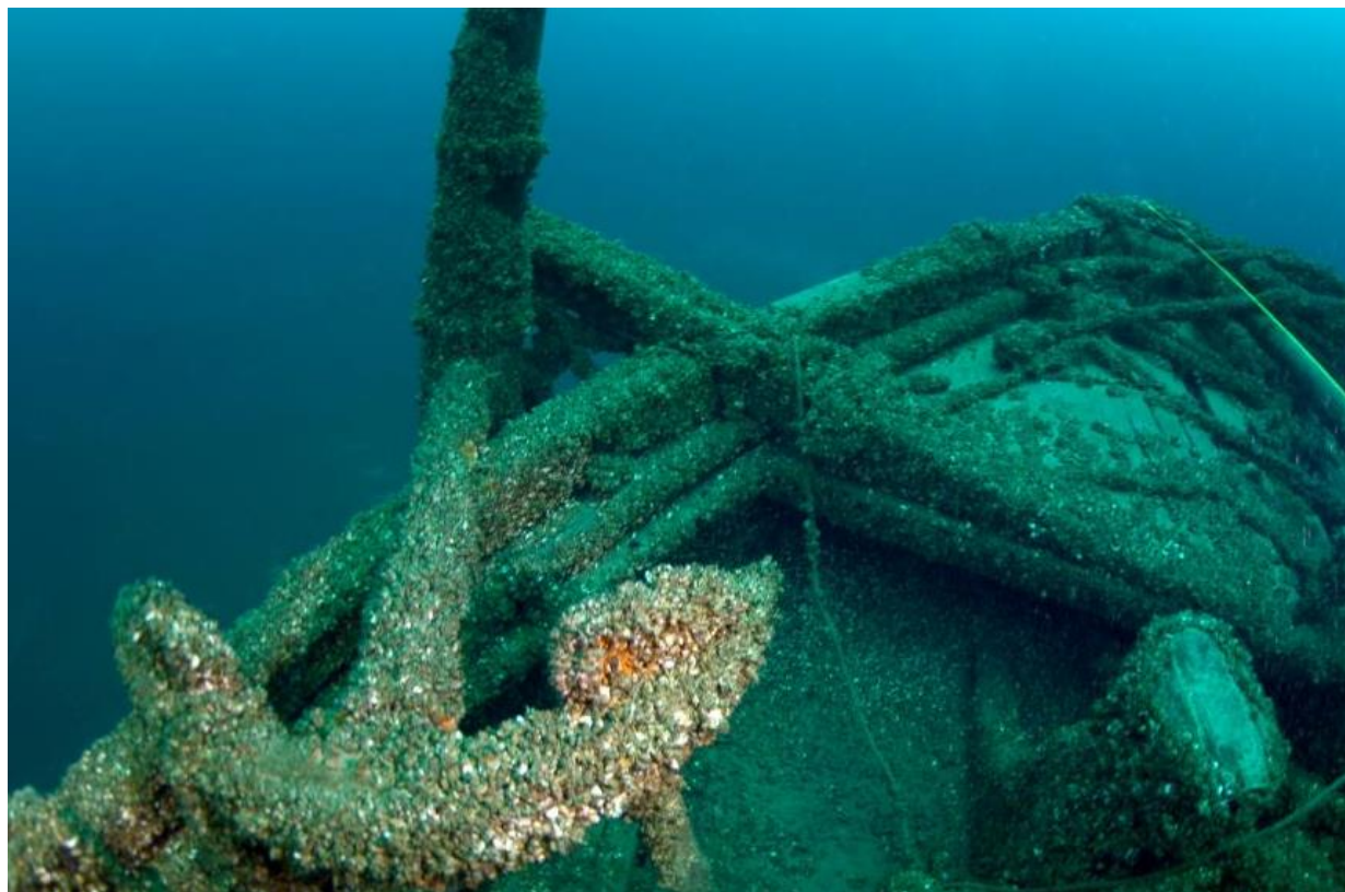
Figure 20: Grace A. Channon 's port side wooden stock anchor and hinged cathead
