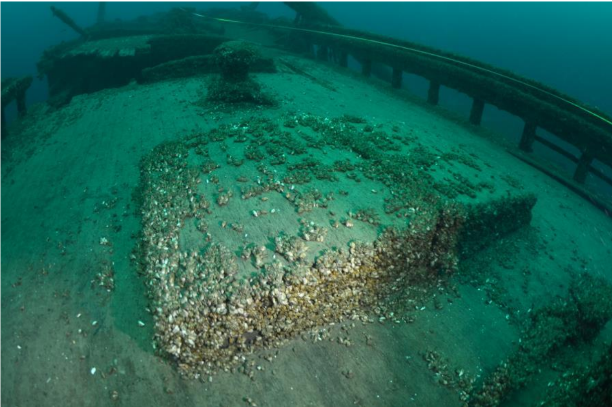
Figure 25. Grace A. Channon 's single, covered cargo hatch
