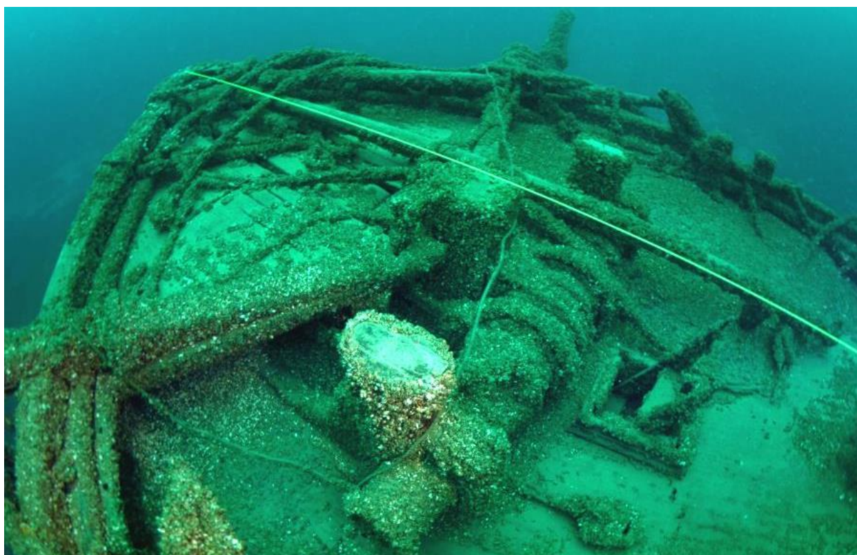
Figure 22. Grace A. Channon 's samson post, windlass and forecastle scuttle
