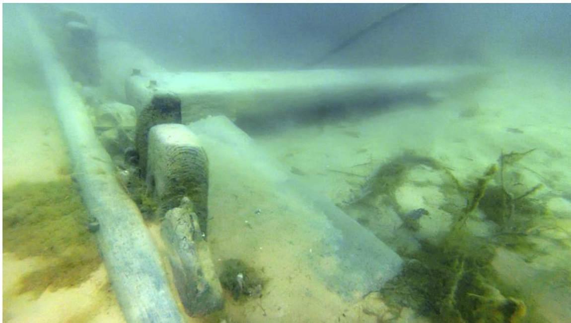
Figure 12: Tubal Cain 's starboard side hull, frames, deck shelf and deck beam (Randy Wallander)
