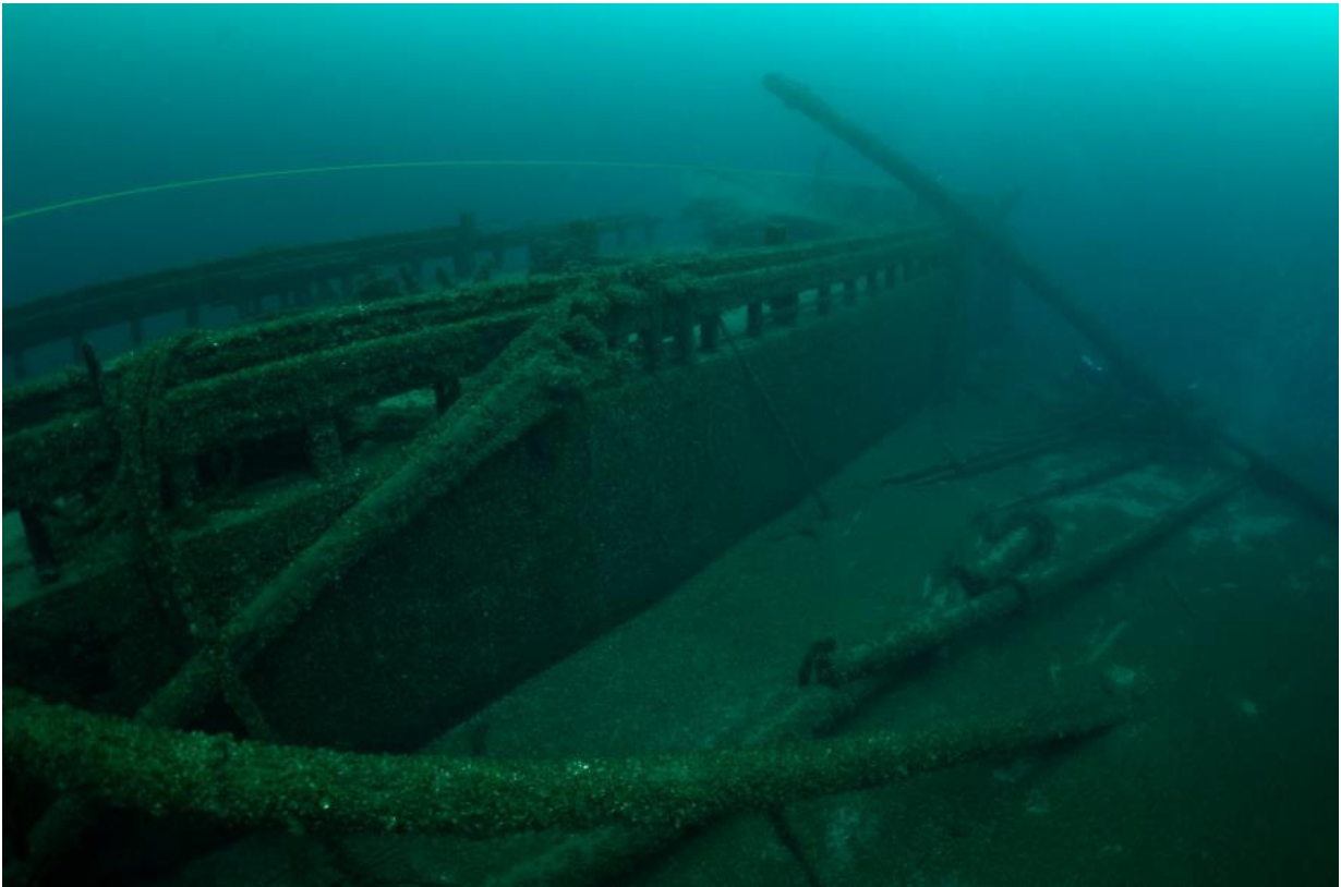
Figure 31. Spars, booms and gaffs on Grace A. Channon 's starboard side
