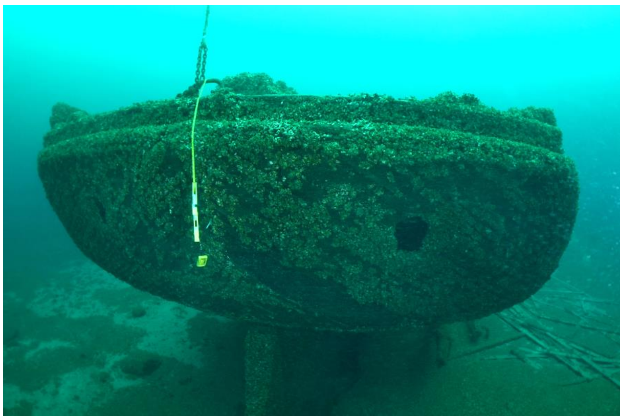
Figure 27. Diagonal decorative planking on Grace A. Channon 's transom
