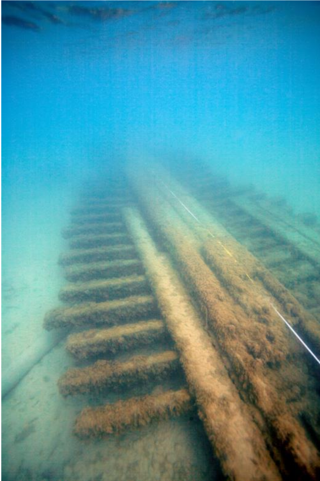
Figure 37. Mainmast step and keelson of H.L. Whitman (Christa Waller)
