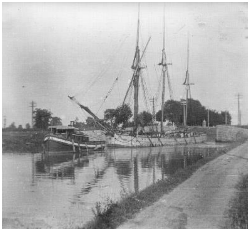
Figure 8. A sailing canaller traversing Lock 4 of the Welland Canal with its bowsprit raised (C. Patrick Labadie Collection)
